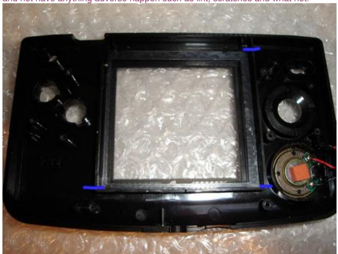
Next you will need to score the left and right walls of the housing. This is done by running your exacto knife along the bottom of the wall from side to side with moderate pressure. You will need to do this about 3 times. Try to score it at the very bottom of the wall as possible as we will be removing these walls to make way for the front light screen.
