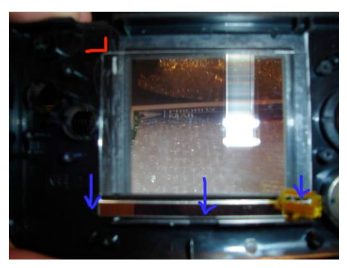
After your front light is in place you will need to place the NGPC LCD back into the housing. YOU WILL need to align the LCD as you no longer have the left and right walls to align it for you. It is simple to do. The upper right wall is still there so you can align it with that. You can also still see where the walls were so don't freak out. Once you align the LCD you can secure it on the left and right sides with electric tape.
