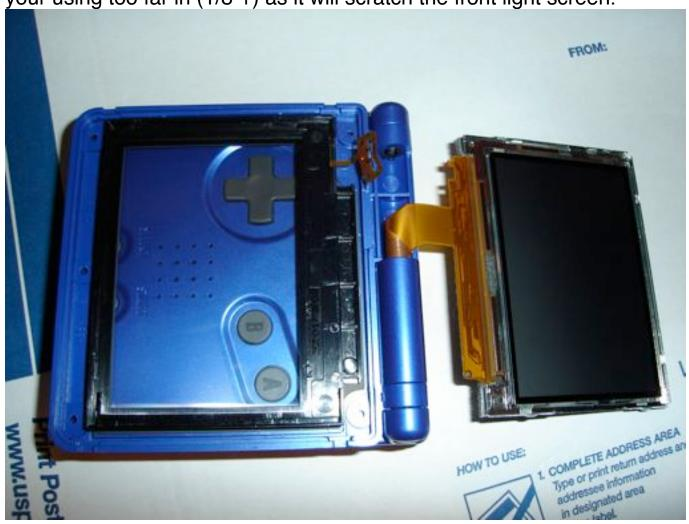
After you remove the LCD you will then need to separate the front light housing from the front plastic screen. This is simply done by gently gliding your exacto knife between the housing and the front plastic screen. Whatever you do, DO NOT touch the front light screen as the oil from your skin will stain the front light screen and if you try to wipe it off it will scratch the front light screen and also transfer lint that you will not be able to remove. The screen is very sensitive.
