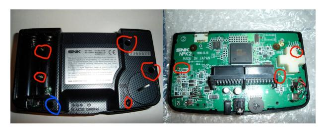
Now you will need to desolder the speaker wiring which are located on the right side of the PCB. Just desolder them and move them out of the way. Next thing you need to do is flip your NGPC over and remove the joystick. This is done by using a flat object to pry it off. I do not use an exacto to do this, it is only for reference. I usually use the flat end of a nail clipper. Insert it from the side and pry it upward so it will slide off, DO NOT force it just be gentle it will slide off.
