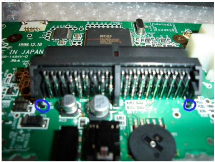
This is also the perfect time to change your Power LED if you want. Simply remove the old one and put the new one in. Remember that the longer lead is the positive and that positive flows to negative (I>), when soldering the new LED in place make sure to raise the LED about 1/8" off the PCB.
