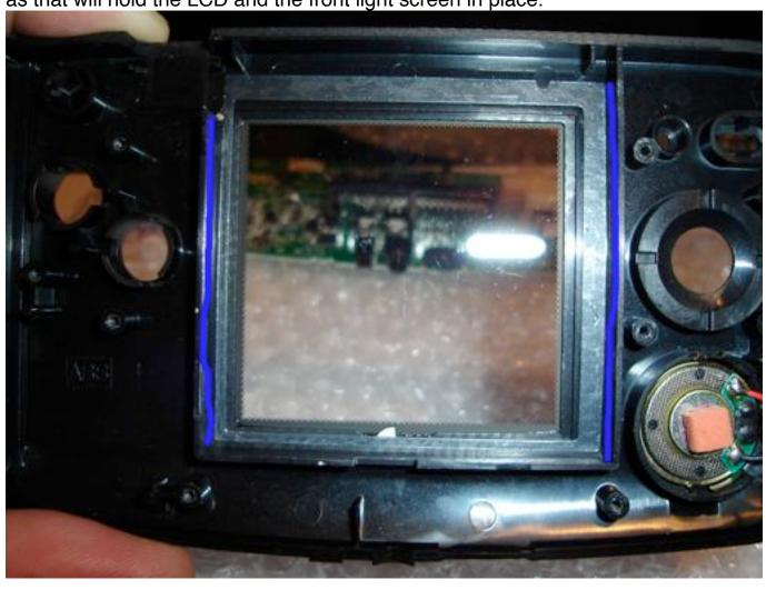
I increased the brightness of this picture so you can see how it should look after you remove the left and right walls. Make sure that there are no peaks in the remnants that are higher than the LCD adhesive. If there is the you will have to flatten them by shaving some plastic off. If there are peaks it will crack the front light screen when the unit is tightened.
