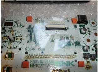
Now you will need to snip off the 4 plastic grommets, these are made to look like they're holding the cartridge slot but since the slot is soldered to the PCB you do not need these. These need to be removed so the front light screen has more space to fit as it is already a tight fit without it. It might be easier to snip them from the back side of the PCB as you may cut a trace from the front side(white).
