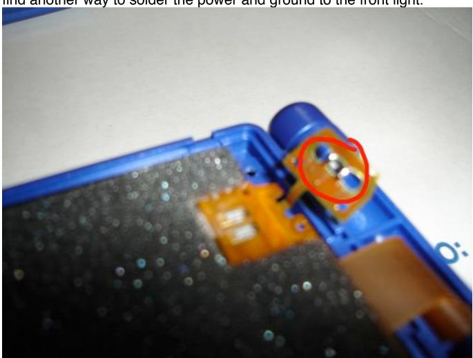
To remove the LCD from the housing just simply pry it out, you will see very small tabs barely holding it in, just pop it out. Do not stick whatever your using too far in (1/8"+) as it will scratch the front light screen.
