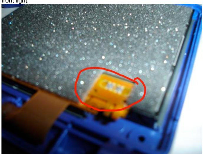
After you desolder the 2 points separate it from the other ribbon, it is imperative that you do not tear this ribbon, if you do you will have to find another way to solder the power and ground to the front light.
