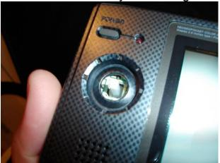
Now with the NGPC screen facing you, you will have to release the LCD ribbon so you can separate the PCB and the front half of the NGPC. This is done in usual ribbon fashion by simply sliding the left and right sides down to unlock it and then
