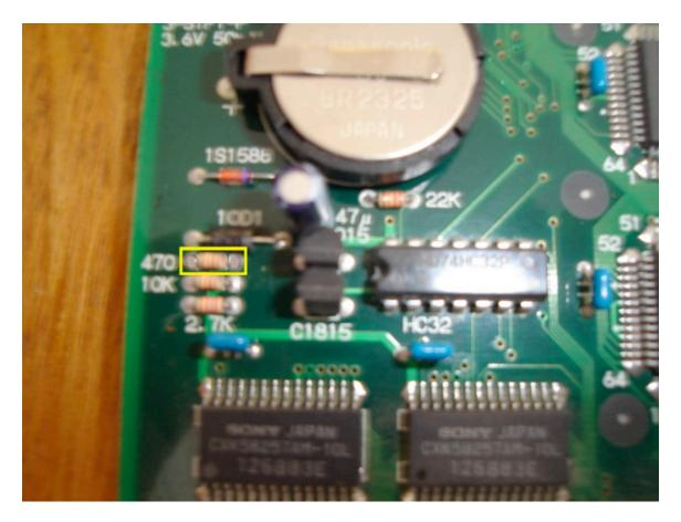
To do this mod all you need to do is remove the 470ohm resistor in this spot:
