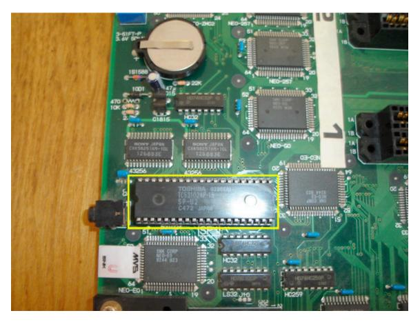
Be very careful when removing the old chip, you can use either a chip puller or a flat head screw driver to remove it. Gently insert the flat head under either side of the chip and GENTLY pry the chip upward about 4mm then repeat on the opposite side. Keep repeating until the chip is out. Once you get the hang of it you will have your own method of removing the old chip.
