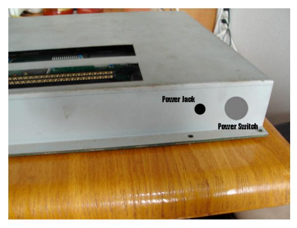
Above is the usual locations that I use for the power jack and the switch. I prefer my 2 slots to have the power switch on the back left side of the unit. To me it is cleaner this way. If you prefer to mount the switch somewhere else go ahead and do it. Just remember that you will need to run some longer wires when you do that.
