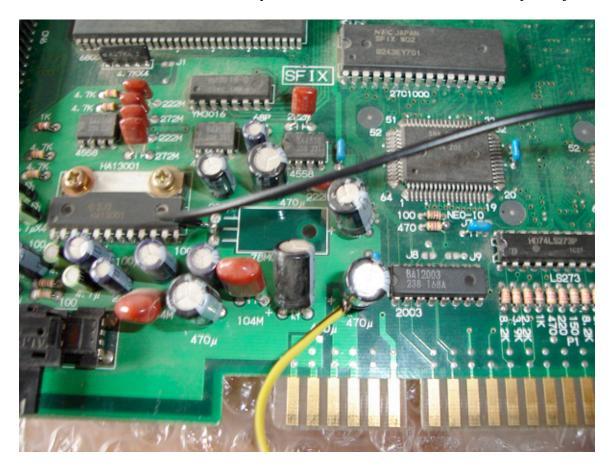
Once you connect the above wires, run the black wire to the ground on the power jack and run the +5v line to the power switch. The power switch is a SPST switch meaning Single Pole Single Throw which is a basic On-Off switch.
