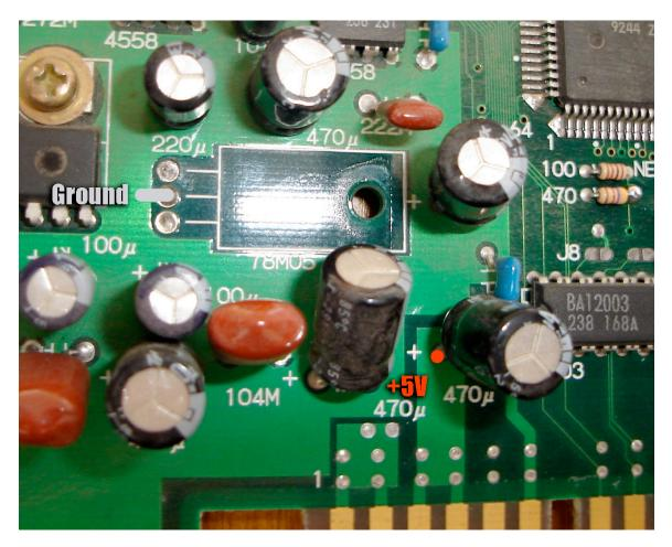
On the other end of the wire you will connect to the power jack. Check your PSU for the polarity. If it says +---(o--- - then you connect the ground to the center pin of the power jack. If it says +---o)---- - then you do the opposite. Pick a spot on the back of the metal casing of the 2 slot to drill the hole for the power jack, power switch and audio and video jacks.
